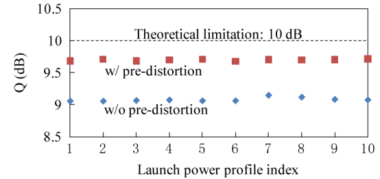
Fig. 11. Q values of ten different launch power profiles. Span number: 25; total length: 1500 km; launch power to each span was randomly in a range from 1.4 to 2.8 mW, keeping the total nonlinear phase shift to be the same.
